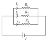
equivalent resistance is given by  $\frac{1}{R_p} = \frac{1}{R_1} + \frac{1}{R_2} + \frac{1}{R_3}$
